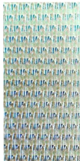
Photo 4: GKD mesh made of PPS for high chemical or thermal loads.
